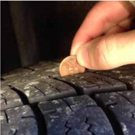
Using a penny to check tires. ©GARRETT LANGER
